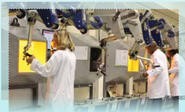
Radiochemical production operations at the NTP hot cell complex
