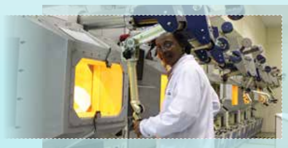
Radiochemical production line in the NTP hot cell complex
