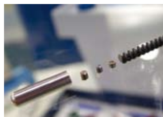
Left: A stainless steel Iridium source capsule assembly, known as a pigtail, contains high purity activated Iridium for industrial radiography.
