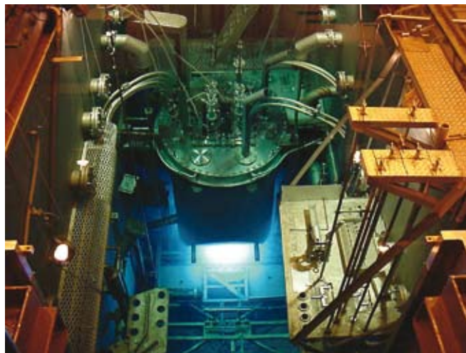
The Safari1 reactor core used for the irradiation of Iridium discs, which are used to produce Ir-192 sealed sources, critical in the field of non-destructive testing.
