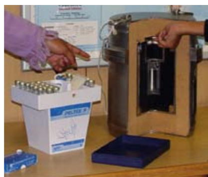
Top: Checking radiation levels in the container closure area. Middle: Preparing chemicals (cold) for use in radiochem production. Above: The radioisotope payload nestles in the centre of the protective container at right; the blue-and-white plastic container at the left is the “generator” that medical technologists use to derive technetium-99 from the molybdenum-99 parent on site.
