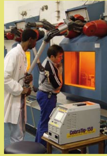
Top: Radiochemical production hot cells. Above: Sealed radioactive source (Ir-192) production. All of these operations take place behind massively thick walls and lead glass. Opposite: The eerie blue glow of the SAFARI-1 nuclear reactor at Pelindaba.
